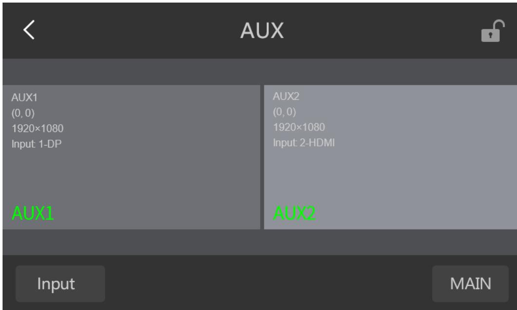
Select an AUX on the touch screen, then tap **Input** or press the corresponding source button in the **SOURCE** area to set the input source for the AUX.
